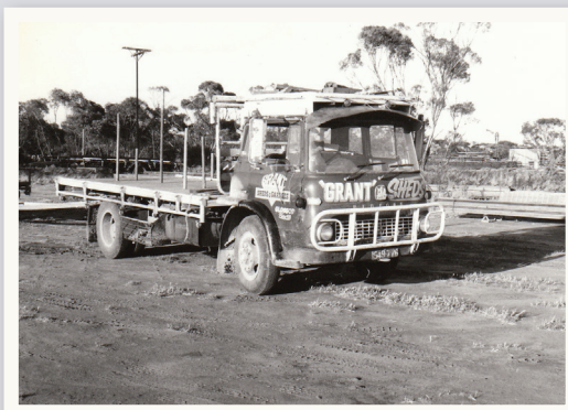
Grant Sheds Bedford 6 ton petrol truck in 1976 (converted to a Perkins diesel power after the petrol engine melted solid out the back of Wentworth).
